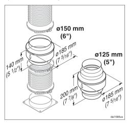
In some cases, a condensate trap may also be required to collect and evaporate any condensate which may occur. This optional accessory is available for ducts 5" (125 mm) and 6" (150 mm) in diameter.
